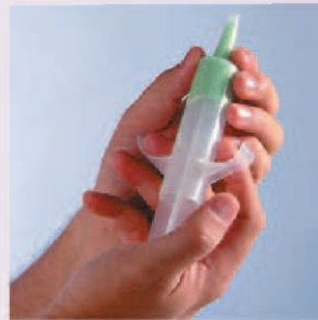
STEP 3 Insert the plunger and force the material to within 1/8" of the end of the nozzle to eliminate air pockets.
